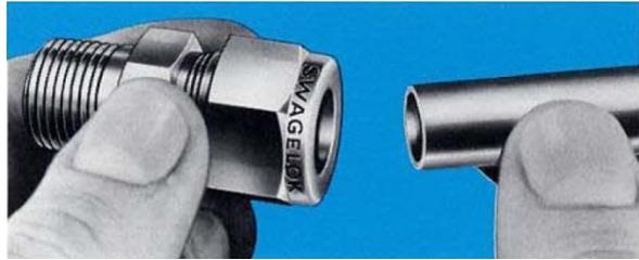
2. Scribe the nut at the 6 o'clock position. By scribing the nut at the 6 o'clock position as it appears to you, there will be no doubt as to the starting position.
