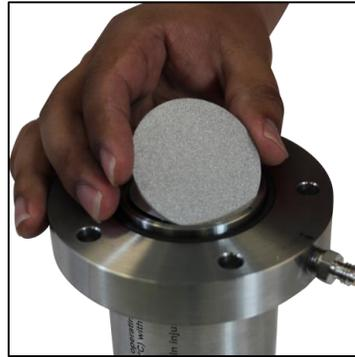
Photo 4: Membrane Support Disk Insertion
