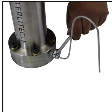
Photo 7: Permeate Tube Installation
