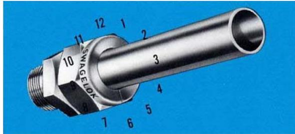
3. Hold the fitting body steady with a backup wrench and tighten the nut  $1\frac{1}{4}$  turns. Watch the scribe mark, make one complete revolution and continue to the 9 o'clock position. When the nut is tightened to the 9 o'clock position, you can easily see the fitting has been tightened properly.
