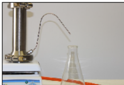
Photo 14: Permeate Collection Vessel
