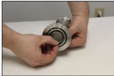
Photo 2: Inner Ring Insertion
