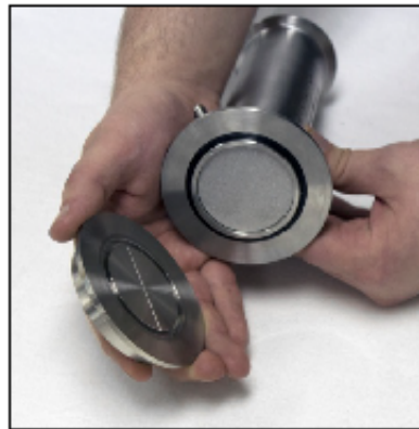
Photo 5: Cell Bottom Assembly
