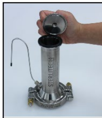
Photo 10: Cell Top Attachment
