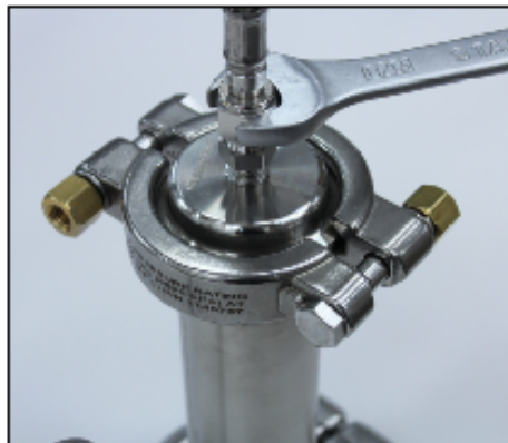
Photo 12: High Pressure Hose Attachment
