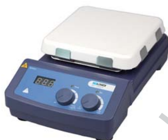
MS7-H550-S LED digital hotplate-stirrer
